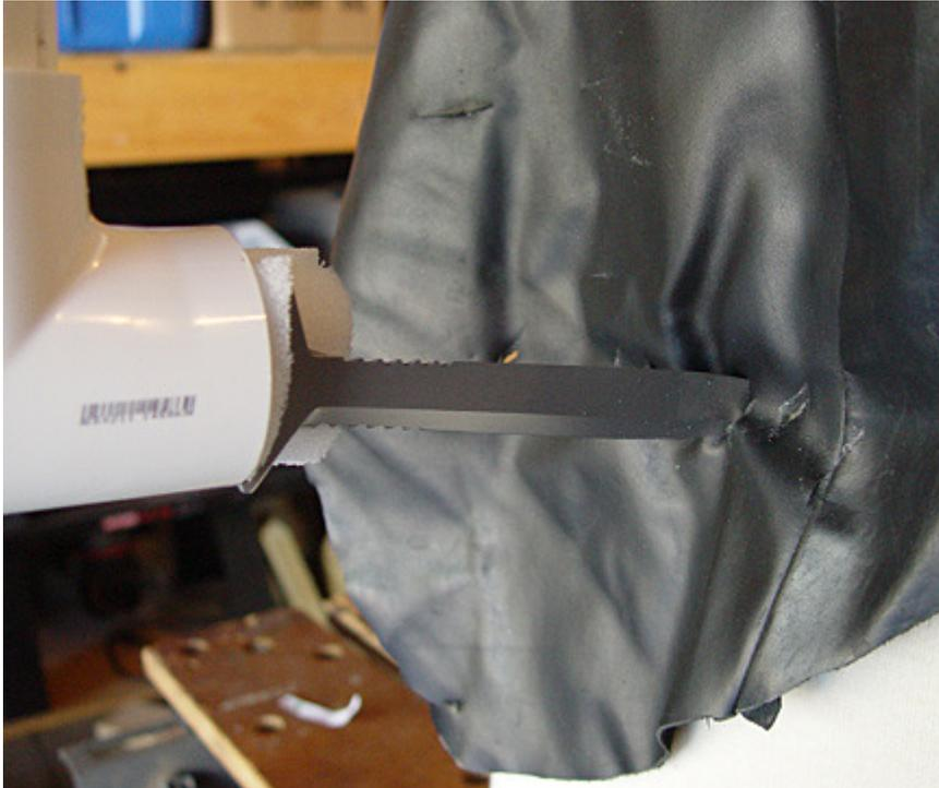
These tests revealed that the XSF-1 consistently penetrated on par with single-edged tantos and traditional Bowie designs, but not quite as well as conventional double-edged daggers. Bear in mind, though, that the XSF-1 also does not suffer from the primary weakness of conventional daggers - a weak and easily broken point. When considered in this context, the extreme durability of the XSF-1's point is much more important than the slightly better penetration offered by traditional daggers.
