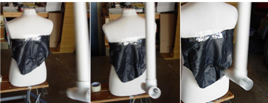
**To scientifically test the penetration performance of the Beshara XSF-1, the author constructed a ballistic pendulum that allowed it to strike a foam torso with uniform force. The results were compared with a variety of other blade and point designs**
