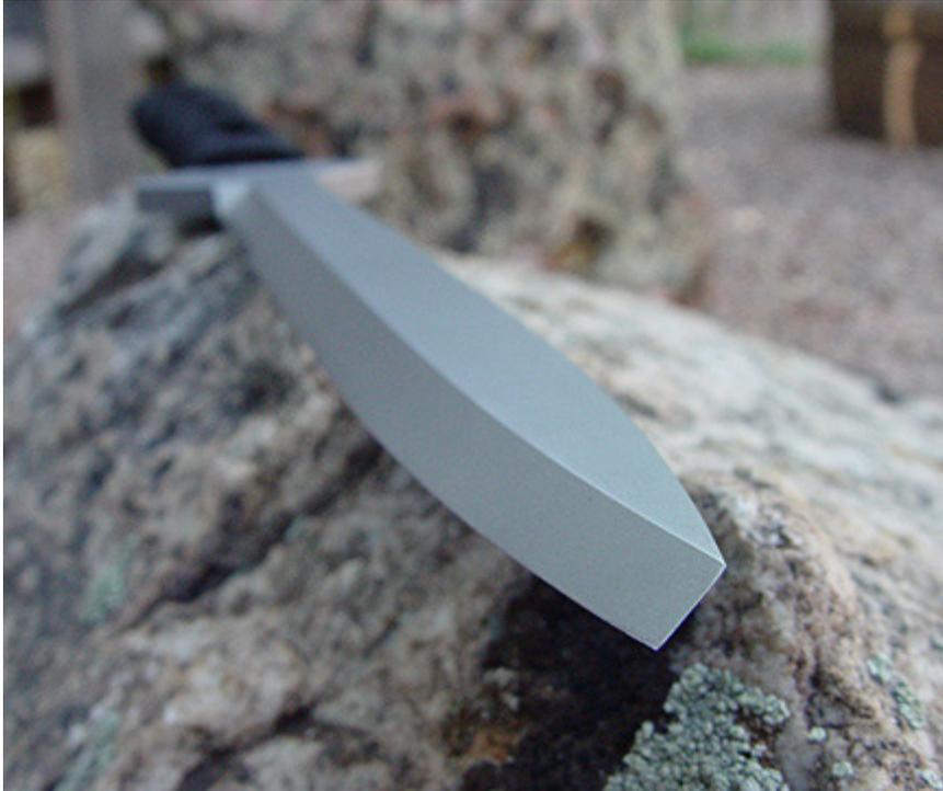
**This view of the XSF-1 shows how its dual chisel grinds converge to form a third cutting edge at the tip of the knife that is substantially stronger than typical dagger points**
